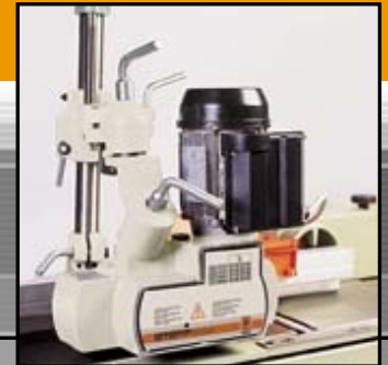
▲ Power feeder positioned on a surface planer
