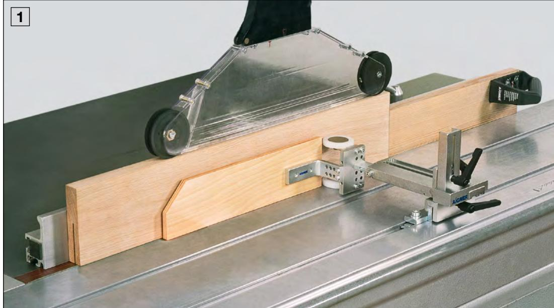
**1** Splitting deep workpieces with a Split-top and pressure module
