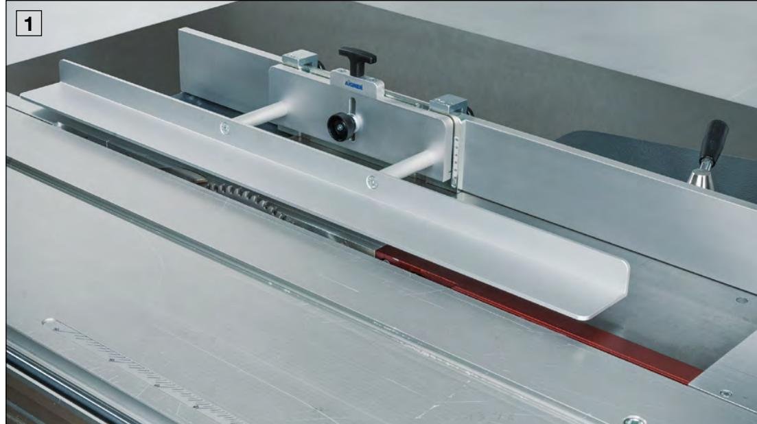
**1** Sawboy mounted to the parallel fence of a Altendorf circular saw.
