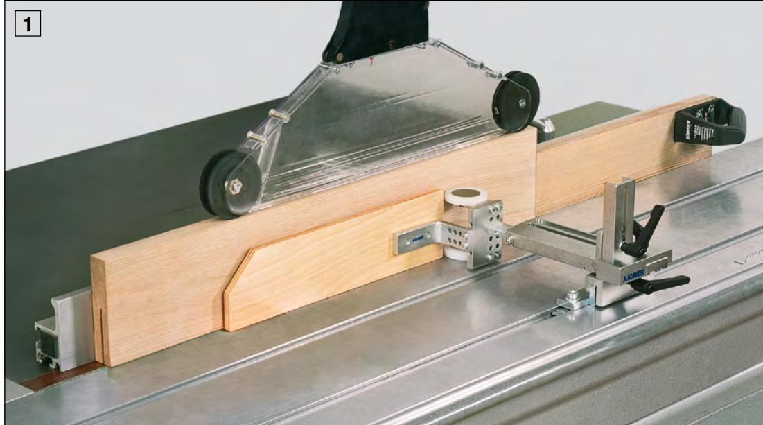
**1** Angle bracket with pressure module
