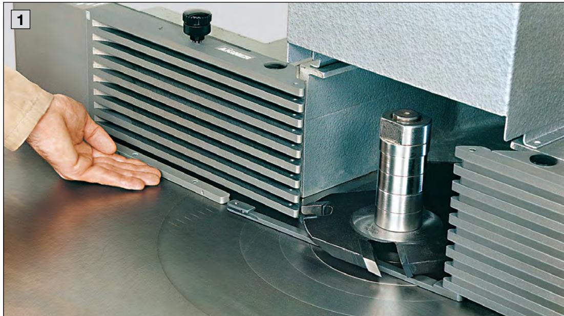
**1** Inserting the filling bar into the lower recess of the outfeed fence case.
