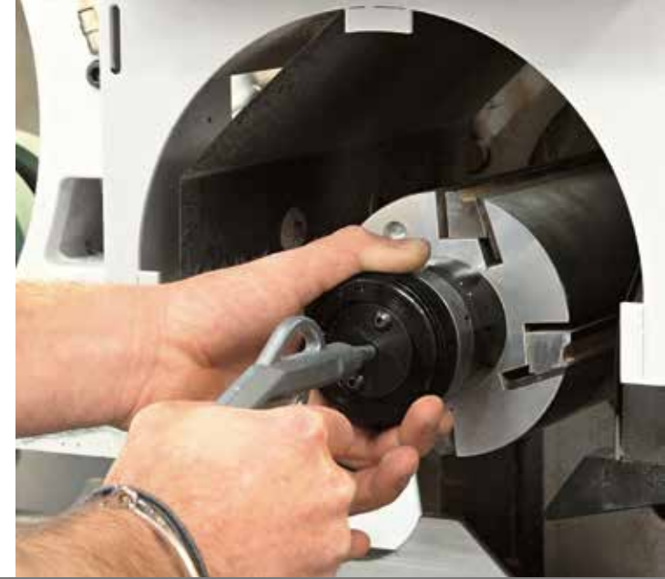
"T-Set": rapid tool locking device It ensures the locking/unlocking of tools simply through a gun with compressed air.
