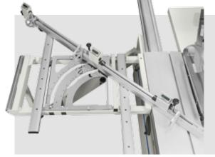
**Compex** To rapidly obtain angular cuttings with automatic self-adjusting of the stop postion.
