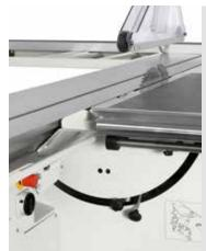
The scoring blade is adjustable from the outside without tools and allows fast and accurate positioning with no play.
