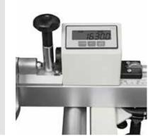
Digital readouts On squaring stops with micrometric adjustment.
