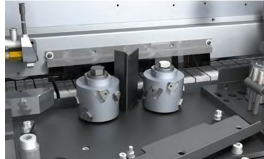
**Pre-milling cutter (WhisperCut):** The WhisperCut jointing system with interchangeable diamond cutting points ensures maximum tool life (manual height adjustment) and tear-free milling results due to an oblique cut through the centre of the panel. Two ready-to-use cutter heads guarantee tear-free milling results, even for demanding materials and surfaces.
