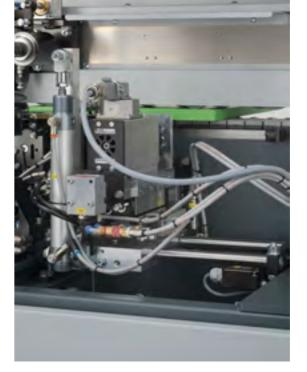
**Corner rounding unit:** Corner rounding optimally prepares you for any challenge when it comes to dealing with the front of the turning heads. Thanks to intelligent programming via the touchscreen display, individual sides and processing settings can be set.
